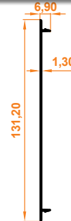
Gizli Ayak ve Destek Kutu Kapatma Profili Hidden Leg Case Cover Support Profile
